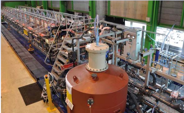
Test of ionic liquid/liquid separator for deep water field realised in cooperation with the Technical Centre of Mechanical Industries (CETIM) of Nantes
