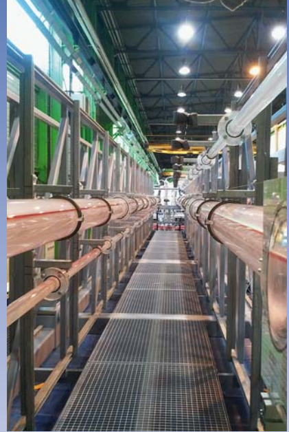
Test of ionic liquid/liquid separator for deep water field realised in cooperation with the Technical Centre of Mechanical Industries (CETIM) of Nantes
